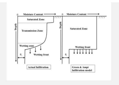
Figure: Soil moisture content distribution in the soil profile modelled by the Green-Ampt model (right) and a typically observed distribution (left) (Neitsch et al., 2011)
